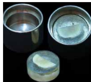
Fig. 3. The specimen and receptacle positioned for simulated toothbrushing.
